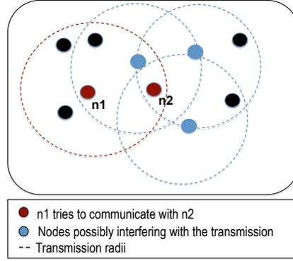
**Figure 9.** Example of interference suffered by a transmission
