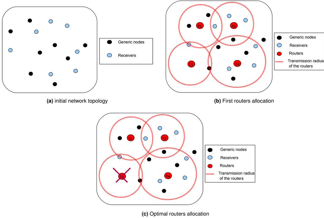
Figure 5. Example of optimized routers allocation
