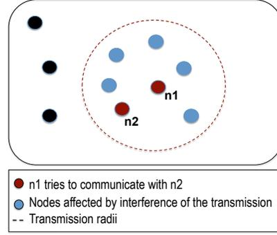
**Figure 8.** Example of interference caused by a transmission
