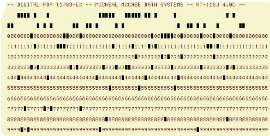
Programs in the 1950s to 1970s are coded on a piece of paper card with punched holes.
