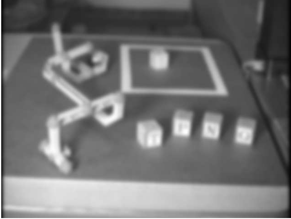
Figure 5: Lowpass filtering (smoothing) an image with a Gaussian filter.
