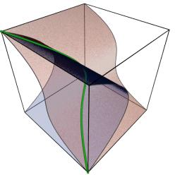
The points all lie on the union of a plane and a single straight line containing the camera center (ie. planar targets won't work!)
