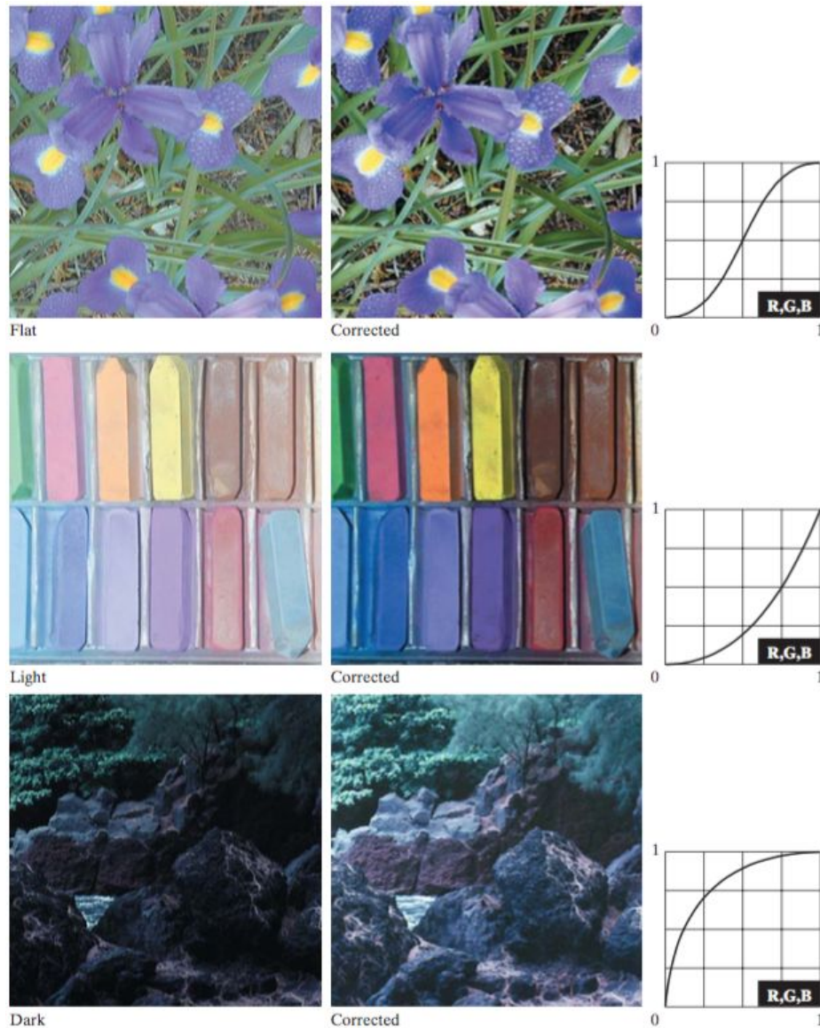
FIGURE 6.35 Tonal corrections for flat, light (high key), and dark (low key) color images. Adjusting the red, green, and blue components equally does not always alter the image hues significantly.
