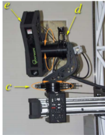
Figure 4: Our laser triangulation scanner and motorized gantry. The scanner, built to our specifications by Cyberware Inc., consisted of an 8-foot vertical truss (a), a 3-foot horizontal arm (b) that translated vertically on the truss, a pan (c) and tilt (d) assembly that translated horizontally on the arm, and a scan head (e) that mounted on the pan-tilt assembly. The scan head contained a laser, range camera, white spotlight, and digital color camera. The four degrees of freedom are shown with orange arrows.
