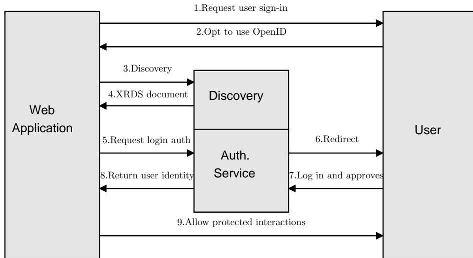
Figure 1: OpenID login authentication for web applications.
