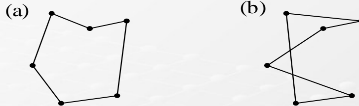
The TSP, showing a good (a) and a bad (b) solution to the same problem
