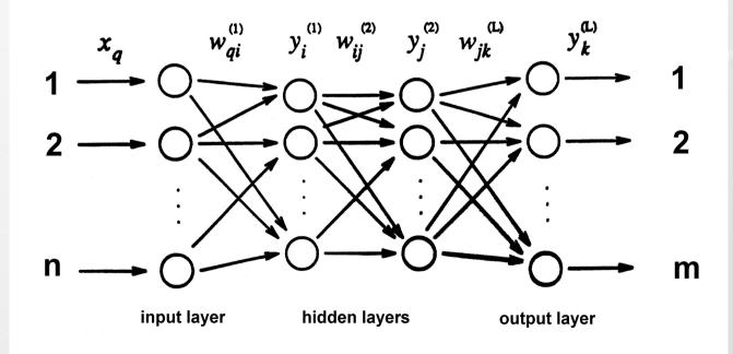
$W_{ij}^{(l)}$ : Weight on connection between the  $i^{th}$  unit in layer (I-1) to  $j^{th}$  unit in layer I
