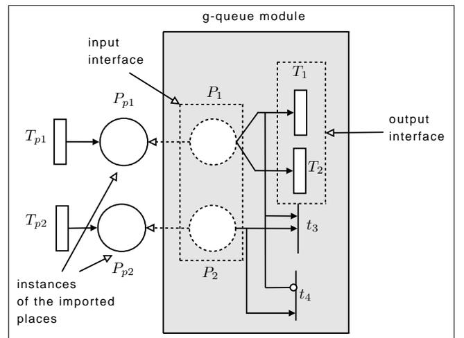
Figure 1: GSPN module equivalent to a G-queue.
