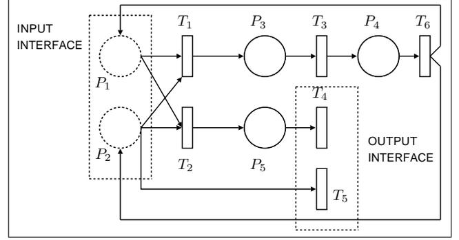
Figure 5: SPN module of the query pre-processing phase.
