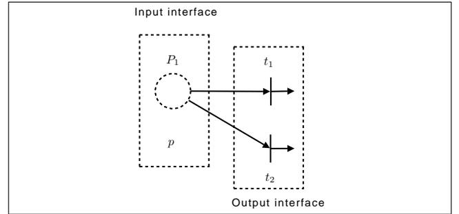
Figure 6: Simple router module. We have  $w(t_1, \cdot) = p$  and  $w(t_2, \cdot) = 1 - p$ .  $\mathcal{I} = \{\chi_{p1}\}$  and  $\mathcal{V} = \{p\}$ .  $f_{M \Rightarrow M} = f_{\text{RCAT}} = \mathbf{true}$  and  $K_1(\mathcal{I}, \mathcal{V}) = p\chi_{p1}$ ,  $K_2(\mathcal{I}, \mathcal{V}) = p\chi_{p2}$ .
