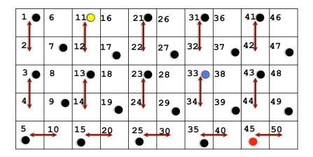
15 mobile, 10 static nodes. Area: 50x100 m. Grid cell: 10x10 m.
